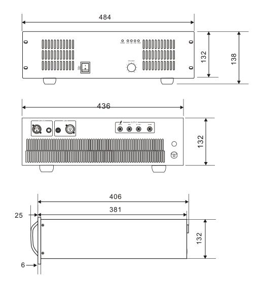
Keep the unit's all sides over 10 cm away from objects that may obstruct air flow to prevent the unit's internal temperature rise.
